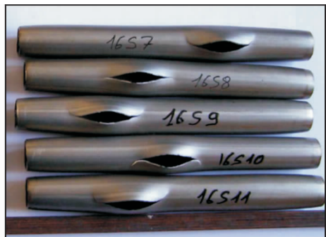
图4 爆破性试验后 \phi 16\text{ mm} \times 0.9\text{ mm} 钛焊管试样照片 Fig. 4 Photos of titanium welded tube specimens ( \phi 16\text{ mm} \times 0.9\text{ mm} ) after blasting test
