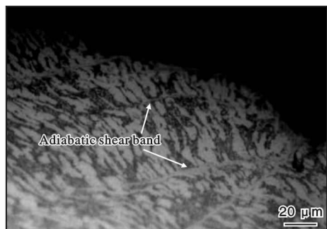
图4 XRF001 钛合金靶板着弹点的绝热剪切带形貌 Fig. 4 Morphology of adiabatic shear band at elastic point of XRF001 titanium alloy target plate
