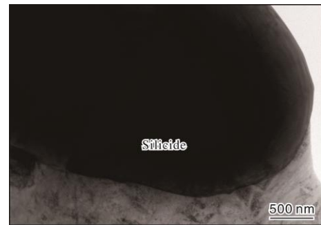
图9 蠕变条件下含3.0% Si元素的Ti6246合金中硅化物形貌 Fig.9 Morphology of silicide in Ti6246 alloy containing 3.0% Si element after creep condition
