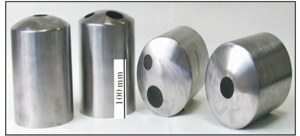
图4 局部加热旋压工艺制备的 Ti-451 合金罐体照片 Fig. 4 Photos of tanks for Ti-451 alloy by local heating spinning process
