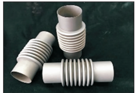
图5 滚珠旋压工艺制备的 CT20 钛合金波纹管 Fig. 5 CT20 titanium alloy corrugated tubes prepared by ball spinning process
